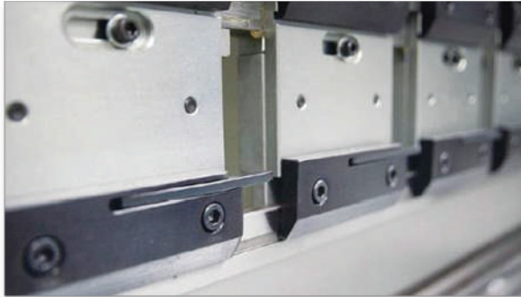
Top and bottom damping system Quick release damping
