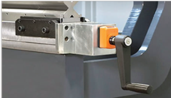
Manual Crowning system - Standard
