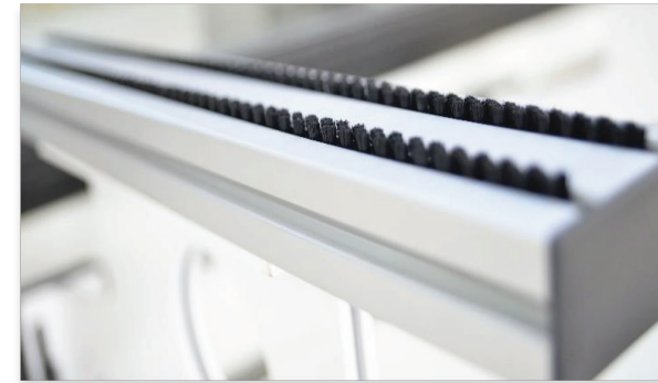
Front support arms with broshes are mounted on a linear guide rail ayatem
