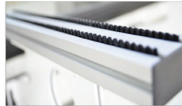
Front support arms with broshes are mounted on a linear guide rail system
